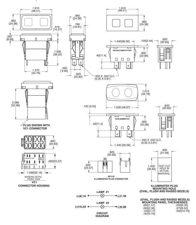
Notes: Oval and flush bezel styles use terminals 1A, 1B, 2A, 2B. Raised bezel style uses terminals 7, 8, 9, 10.
