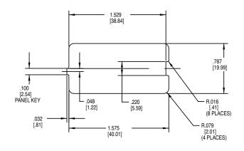
PANEL THICKNESS: 2.5±0.1mm PANEL OPENING CLEARANCE: ±5° SCALE 2.000
